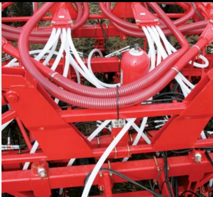
Down force can be adjusted from 200 to 690 lbs depending on spacing and available frame weight
