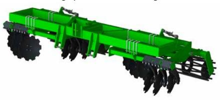
The TrackAttack® by K-Line Ag is designed to level out wheel tracks, ruts and uneven terrain. The front row of discs cut through the ground, loosening and moving the soil onto the tram-line, then the crumbler roller follows behind breaking down the soil and cloddy dirt. This leaves the tram-line with a flat and even weed free surface, making it easier and smoother for equipment to pass.
