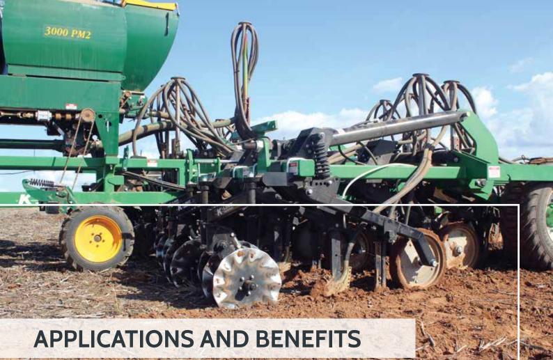
A significant advantage of K-Line Easy Fit Coulter Kits is that they speed up the sowing process by preparing the way for the tine to pass through the soil and minimising trash entanglement. Without a coulter to aid this process, a tine will cause excessive soil disturbance when breaking through the soil, which results in trash blockages and an uneven seedbed.
